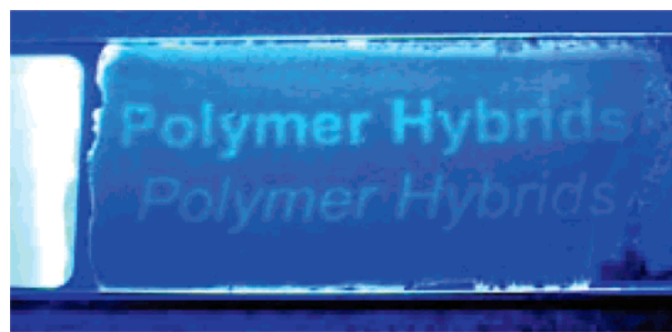
Figure 5. Picture of the transparent hybrid film (run 8) after UV (300 nm) irradiation with photomask.
